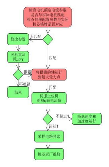
刹车故障导致电机过载问题排查:
